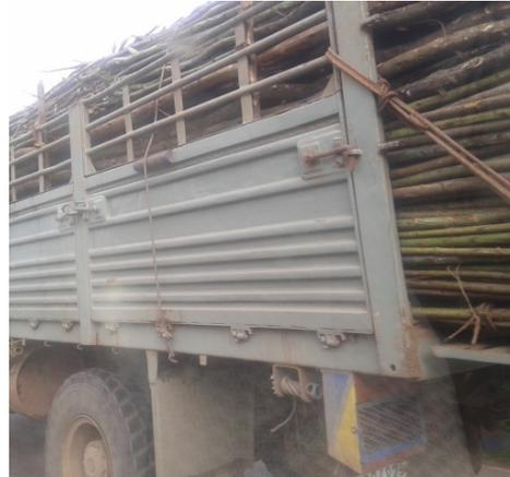
Figure 3: A truck load of tree poles on the road to Addis Ababa. The building construction industry absorbs them for scaffolding. Photo credit: Author
