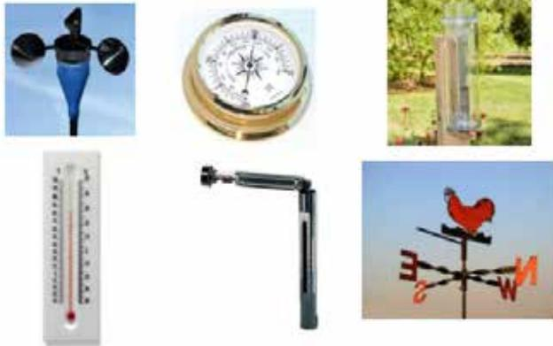
**Figure 67. Tools and instrumentation.**
