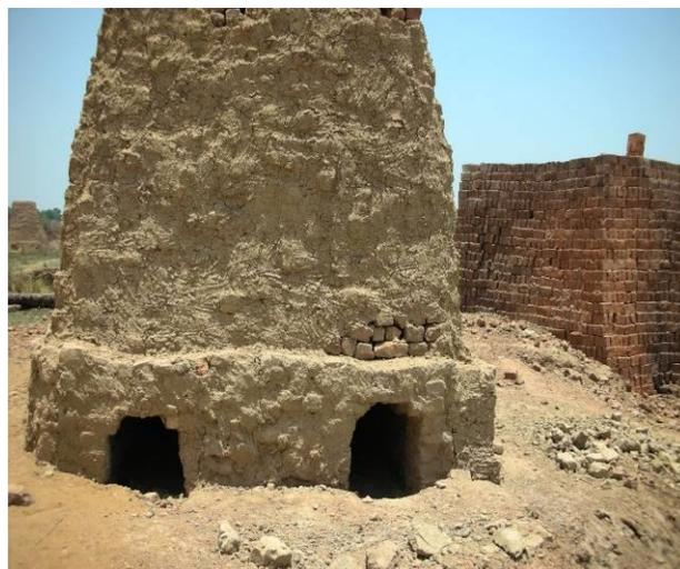
**Figure 10. Charcoal making kiln in semi-arid setting: western Burkina Faso.**
